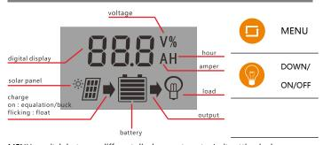
MENU: switch between different display, or to enter/exit setting by long press. DOWN:press to decrease value.
